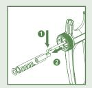
Mount plunger in barrel. Connect rod.
